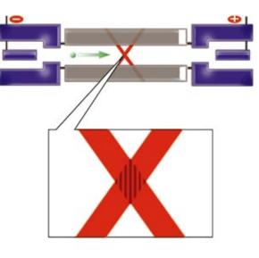
The sample under investigation is contained within an electrophoresis cell. A known field is applied and the sample illuminated by crossed focused laser beams.
